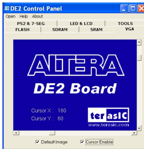
Figure 3.9. Displayed image and the cursor controlled by the scroll bars
